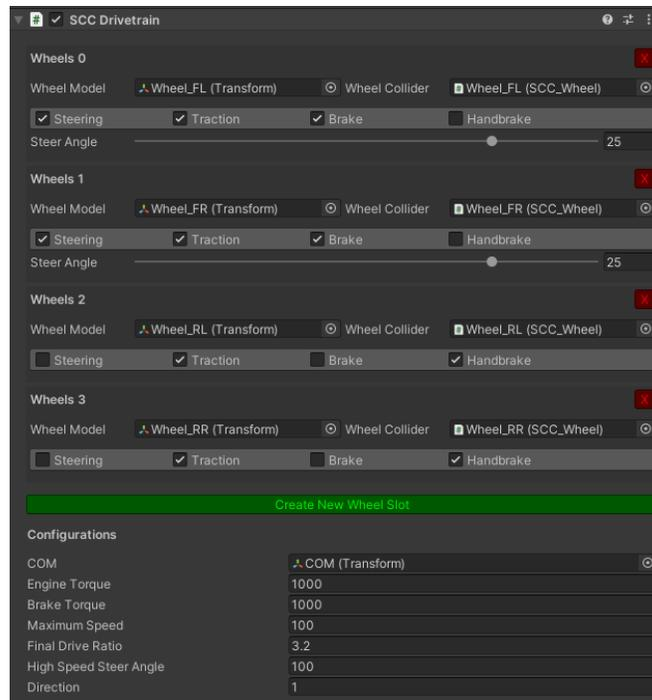
You can set steer, traction, brake and handbrake states of the wheels independently. **COM** (Center of mass) position will be created automatically, but you need to set it manually. You can check the demo vehicles. If you please **COM** too high, vehicle will roll to the sides easily.
